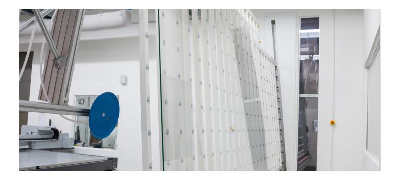
A specially developed tilting table swivels glass panels from vertical to horizontal.
