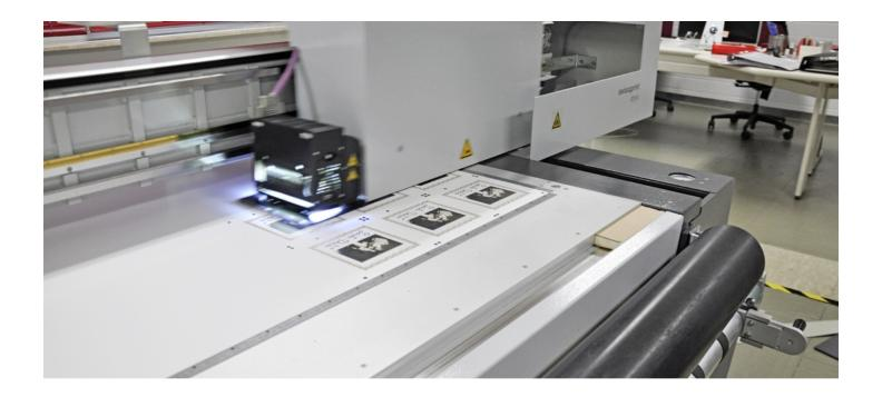
The Oryx UV printing machine appeals with precise printing, and requires only a modest amount of space. The Bräutigam: Medien team uses it for any and all kinds of printing jobs required in developing sophisticated packaging prototypes.
