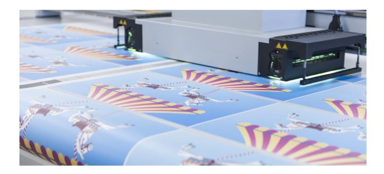
Two rolls of posters loaded up in parallel halve production time for roll printing.
