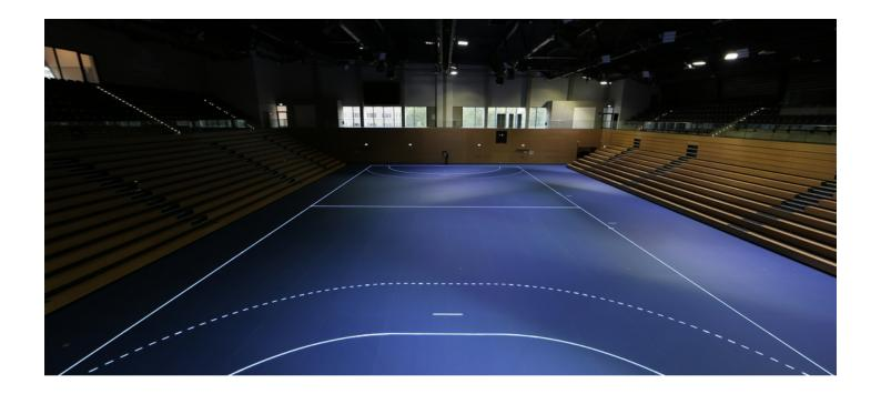
No more confusing jungle of lines in sports halls: printed glass flooring with backlit pitch markings. (Image by ASB)
