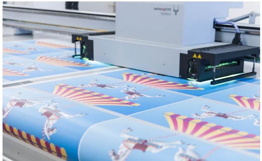
Two strips of posters loaded up in parallel halve production time for roll printing.
