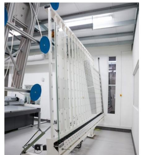
A specially developed tilting table swivels glass panels from vertical to horizontal.
