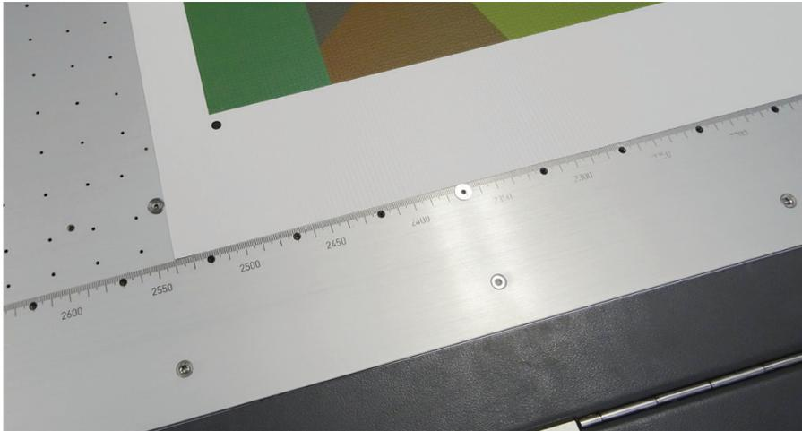
Registration pins do valuable service, especially with the flip function. In general, they ensure a precise registration and help to make full use of the print bed.
